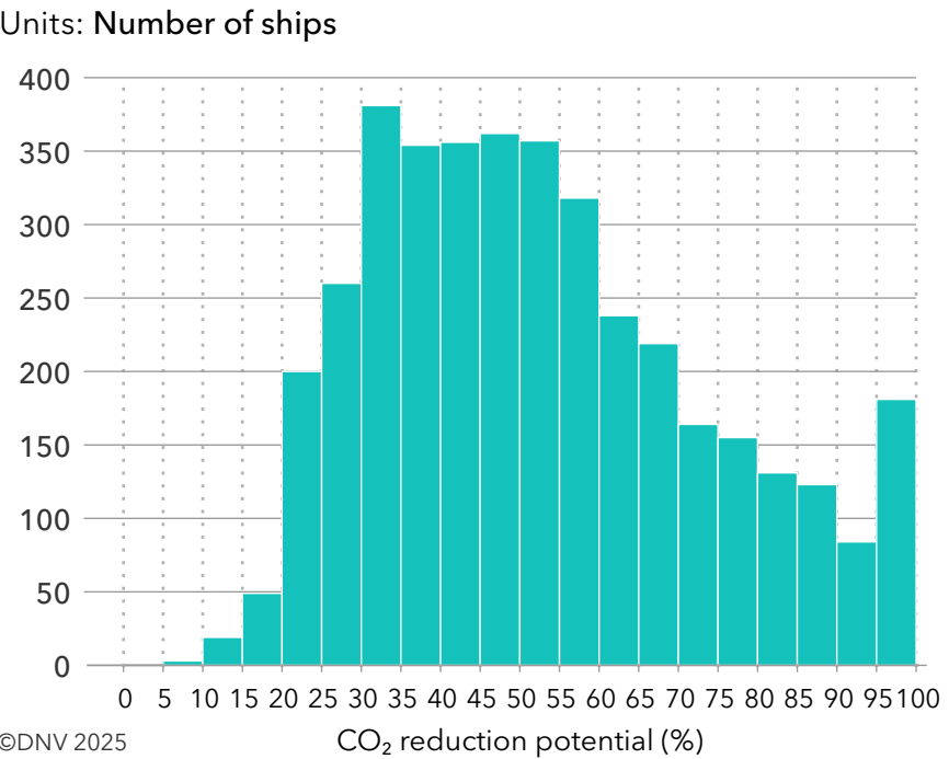
FIGURE 7-4 Number of containerships above 2 000 TEU (3 954 ships in total) with different annual CO 2 reduction potentials from onboard CO 2 capture, assuming given tank volumes and 100% capture rate
